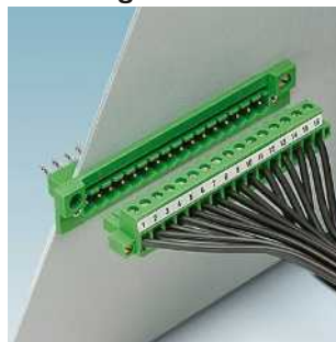
Headers for panel feed-through, 5.0/5.08 mm pitch, with spade connection DFK-MSTB 2,5/...-G(F)-... Page 352
