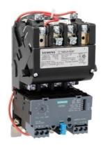
Non-reversing motor starter Size 2 Three phase full voltage Solid-state overload relay OLRelay amp range 13-52a 240VAC 50HZ / 277VAC 60HZ coil Combination type No enclosure
