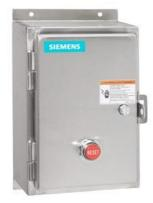
Non-reversing motor starter, Size 1, Three phase full voltage, Solid-state overload relay, OLR amp range 10-40A, 24VAC 50-60Hz coil, Non-combination type, Encl. type 4X 304 S. Steel, Water/dust tight noncorrosive, Extra-wide enclosure
