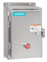
Non-reversing motor starter, Size 0, Three phase full voltage, Solid-state overload relay, OLR amp range 0.75-3.4A, Non-combination type, Encl. type 4X 304 S. Steel, Water/dust tight noncorrosive, Standard width enclosure
