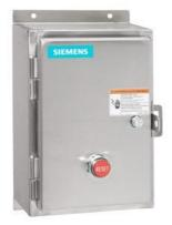
Non-reversing motor starter, Size 0, Three phase full voltage, Solid-state overload relay, OLR amp range 0.75-3.4A, 110V 50Hz / 120V 60Hz coil, Non-combination type, Encl. type 4X 304 S. Steel, Water/dust tight noncorrosive, Standard width enclosure
