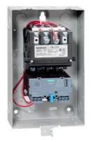
Non-reversing motor starter, Size 00, Three phase full voltage, Solid-state overload relay, OLR amp range 3-12A, 240V 50Hz / 277V 60Hz coil, Noncombination type, Enclosure type 1, Indoor general purpose use, Standard width enclosure
