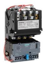
Non-reversing motor starter Size 00 Three phase full voltage Solid-state overload relay OLRelay amp range 0.75-3.4A 24Vdc coil Combination type No enclosure
