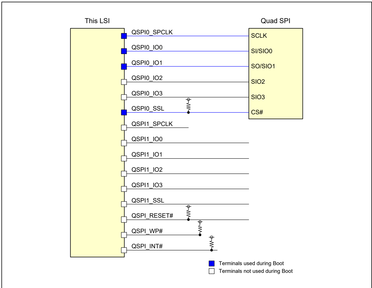
Figure 4.12 Connections with Quad SPI Memory in Boot Mode 3
