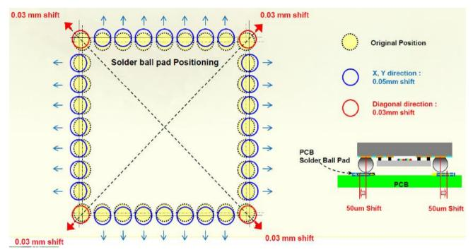
Figure 16: Recommended solder ball pad shift
