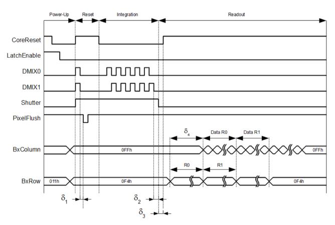
Figure 7: Global shutter timing  $\delta 1 \ge 0.1$ us,  $\delta 2 \ge 0.1$ us,  $\delta 3 \ge 1$ us,  $\delta 4 \ge 1$ us. Each cycle consists of a reset phase, an integration phase and a read-out phase.
