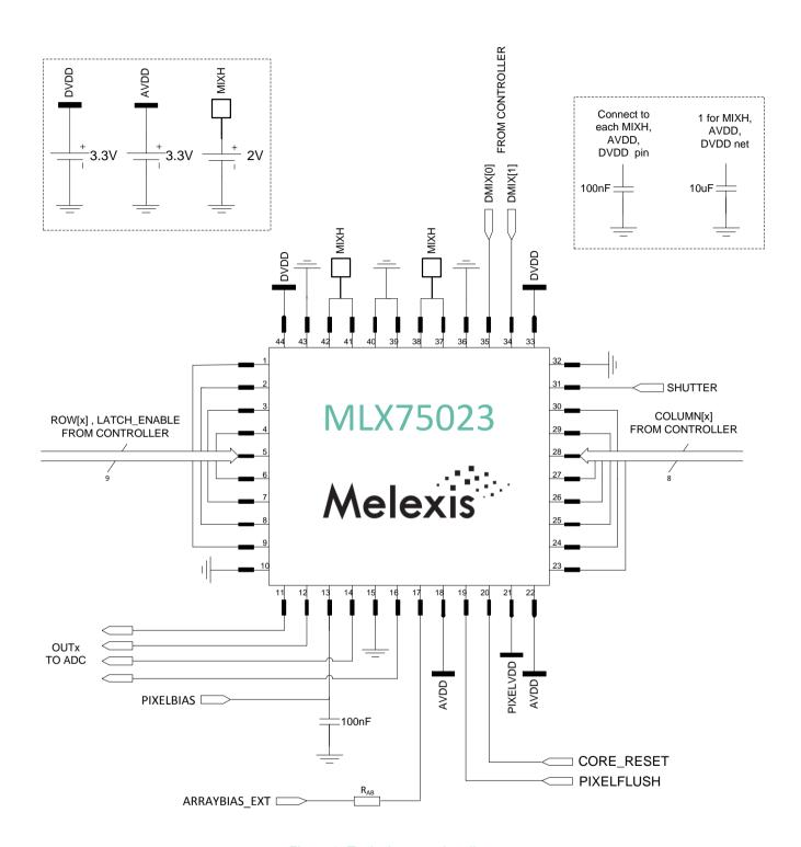
Figure 3: Typical connection diagram
