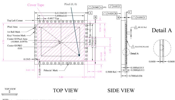
DIMENSION IS MEASURED AT THE MAXIMUM SOLDER BALL DIAMETER, PARALLEL TO PRIMARY DATUM C. PRIMARY DATUM C AND SEATING PLANE ARE DEFINED BY THE SPHERICAL CROWNS OF THE SOLDER BALLS.
