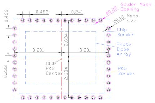
Figure 17: Recommended PCB land pattern (dimenions in mm)
