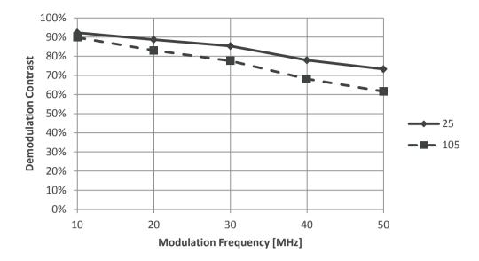
Figure 5: Typical AC demodulation contrast versus modulation frequency at T<sub>a</sub> 25°C and 105°C, 1.5V VMIXH, 0V PIXELBIAS, -3.3V ARRAYBIAS\_EXT, 330 Ohm R<sub>AB</sub>
