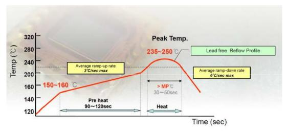
Figure 19: Recommended reflow profile
