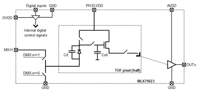
Figure 11: Electrical model of one phase output of the pseudo differential TOF pixel
