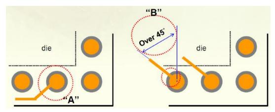
Figure 18: Recommended trace layout
