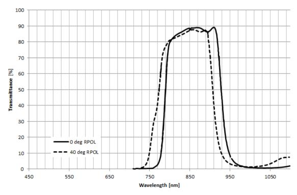
Figure 14: Bandpass filter spectral response for 0° and 40° angle of incidence (AOI)
