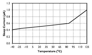
Figure 3. Sleep Current Variation over Temperature, V<sub>DD</sub> at 3.3V
