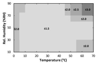
Figure 5. HS3101-MCx RH Accuracy over Temperature
