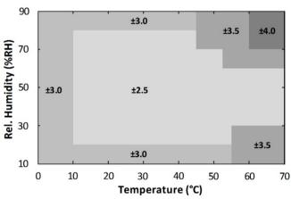
Figure 7. HS3103-MCx RH Accuracy over Temperature
