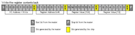
Figure 15. Sequence of Commands to Change the Relative Humidity Resolution
