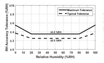
Figure 6. HS3103-MCx RH Accuracy Tolerance at 25°C
