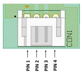
Figure 1. Pin Assignments
