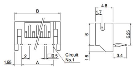
Figure 2. Pin Connector
