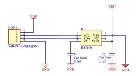
Figure 16. HS310x-MCx Application Circuit
