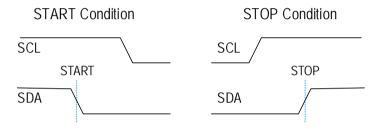
Figure 11. START and STOP Condition Waveform
