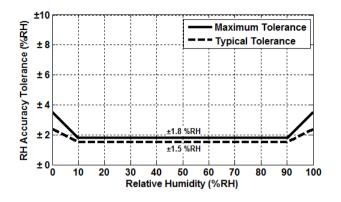
Figure 4. HS3101-MCx RH Accuracy Tolerance at 25°C
