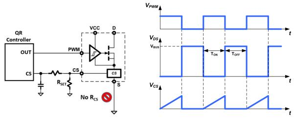
Fig. 26. Current sensing circuit and timing diagram
