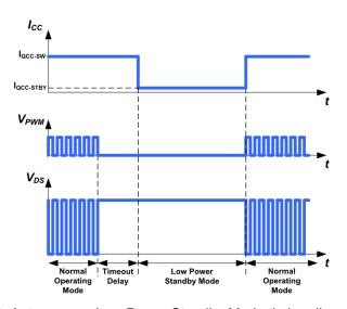
Fig.24. Autonomous Low Power Standby Mode timing diagram
