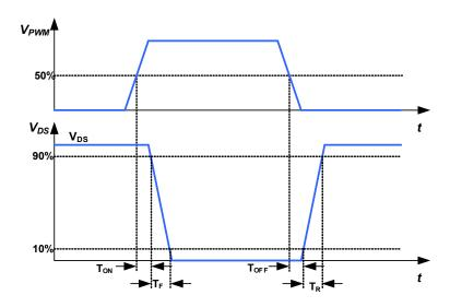
Fig. 1. Propagation Delay and Rise/fall Time Definition
