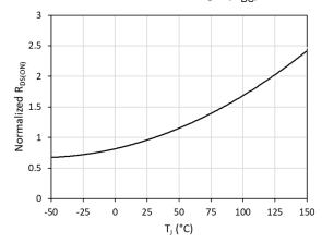
Fig. 7. Normalized on-resistance  $(R_{DS(ON)})$  vs. junction temperature  $(T_J)$
