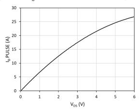
Fig. 2. Pulsed Drain current ( $I_D$  PULSE) vs. drain-to-source voltage ( $V_{DS}$ ) at T = 25 °C
