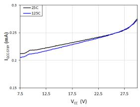
Fig. 13. V<sub>CC</sub> stand-by quiescent current (I<sub>QCC</sub>) vs. supply voltage (V<sub>CC</sub>)
