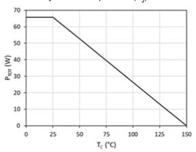
Fig. 16. Power dissipation ( $P_{TOT}$ ) vs. case temperature (T<sub>C</sub>)
