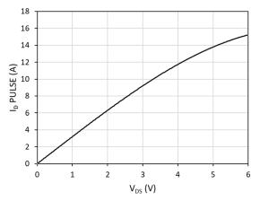
Fig. 3. Pulsed Drain current ( $I_D$  PULSE) vs. drain-to-source voltage ( $V_{DS}$ ) at T = 125 °C
