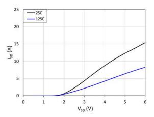
Fig. 4. Source-to-drain reverse conduction voltage
