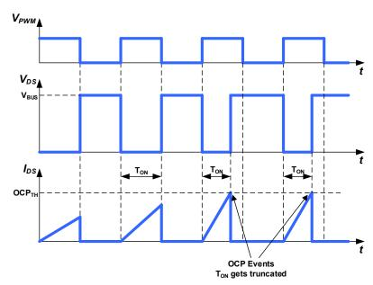
Fig. 28. OCP threshold timing diagram
