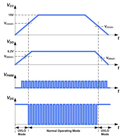
Fig. 22. UVLO Mode timing diagram
