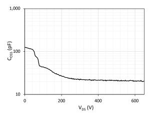
Fig. 8. Output capacitance ( $C_{OSS}$ ) vs. drain-to-source voltage ( $V_{DS}$ )
