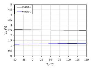
Fig. 6.  $V_{\text{LOGIC-H}}$  and  $V_{\text{LOGIC-L}}$  vs. junction temperature  $(T_{\text{J}})$
