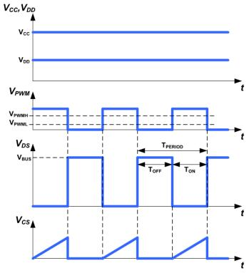
Fig.23. Normal operating mode timing diagram
