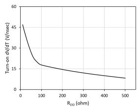
Fig. 15. Slew rate (dV/dt) vs. gate drive turn-on current set resistance ( $R_{\rm DD}$ ) at T = 25 °C
