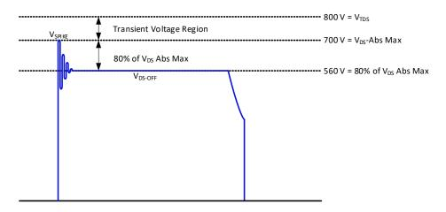
Fig.30. QR flyback drain-to-source voltage stress diagram
