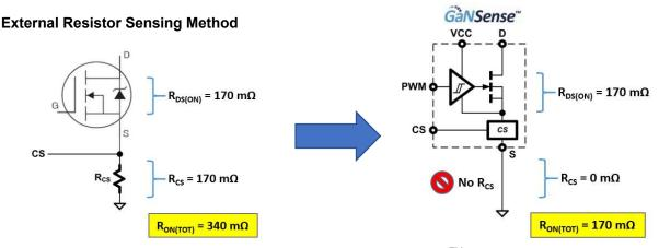
Fig. 27. External resistor sensing vs. GaNSense™ Technology
