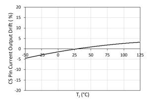
Fig. 18. CS Pin Current Output Drift vs. case temperature (T<sub>C</sub>)
