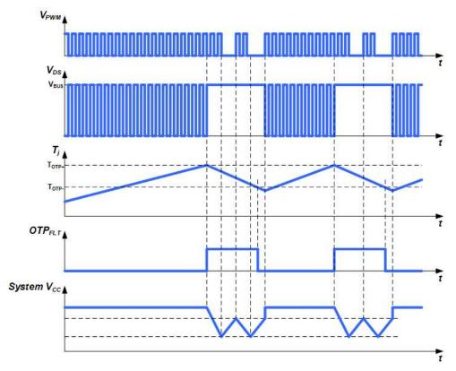
Fig. 29. OTP threshold timing diagram
