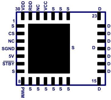
Fig. 19. Package Top View
