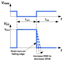
Fig. 25. Turn-on dV/dt slew rate control
