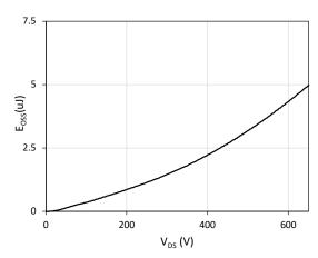
Fig. 9. Energy stored in output capacitance ( $E_{\rm OSS}$ ) vs. drain-to-source voltage ( $V_{\rm DS}$ )
