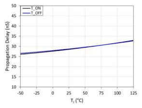
Fig. 14. Propagation delay (T $_{\rm ON}$  and T $_{\rm OFF}$ ) vs. junction temperature(T<sub>1</sub>)
