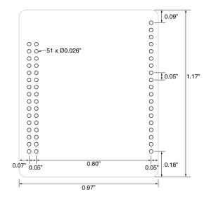
Figure 6: EVM-fff-PRC-CAS and EVM-fff-PRC-UFL PCB Layout Dimensions
