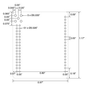
Figure 5: EVM-fff-PRC PCB Layout Dimensions
