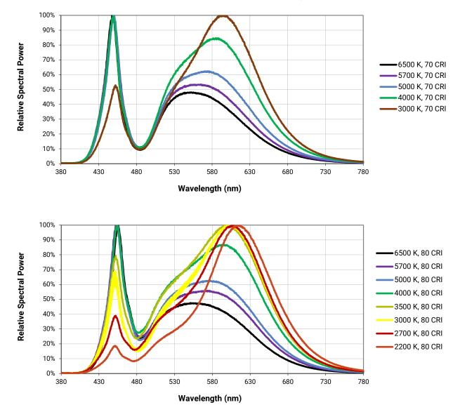
The following graphs are the result of a series of pulsed measurements at 1100 mA and  $T_{J}$  = 85 °C.
