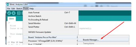
Once the Board Manager opens, click on the category drop down menu on the top left hand side of the window and select Contributed. You will then be able to select and install the boards supplied by the URLs added to the prefrences. In the example below, we are installing support for Adafruit AVR Boards, but the same applies to all boards installed with the Board Manager.
