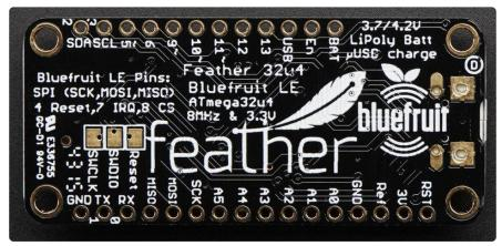
The DFU pin is accidentally labeled GND on the bottom, sorry about that! it should be labeled DFU, dont use it as a GND
