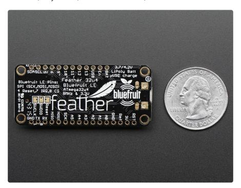
To make it easy to use for portable projects, we added a connector for any of our 3.7V Lithium polymer batteries and built in battery charging. You don't need a battery, it will run just fine straight from the micro USB connector. But, if you do have a battery, you can take it on the go, then plug in the USB to recharge. The Feather will automatically switch over to USB power when its available. We also tied the battery thru a divider to
