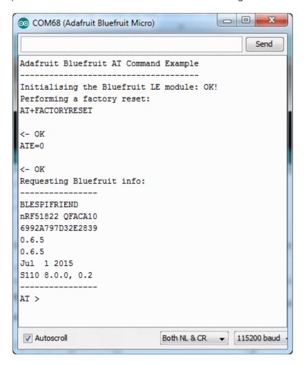
This sketch starts by doing a factory reset, then querying the BLE radio for details. These details will be useful if you are debugging the radio. If you see the information as above, you're working! (Note that the dates and version numbers may vary)
