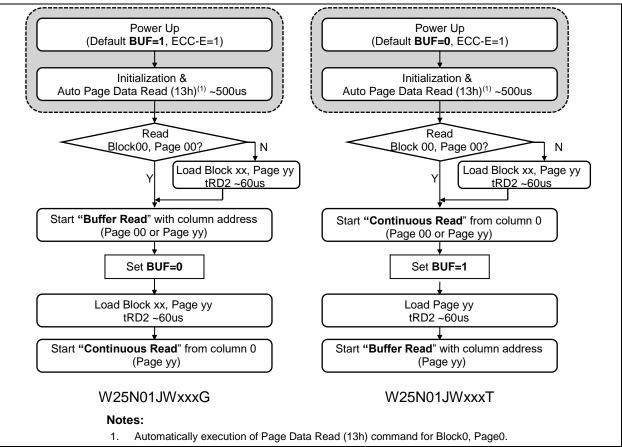
Figure 6-1 W25N01JW Flash Memory Operation Diagram
