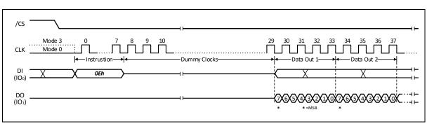
Figure 8-43 DTR Fast Read with 4-Byte Address Instruction (Buffer Read Mode, BUF=1)
