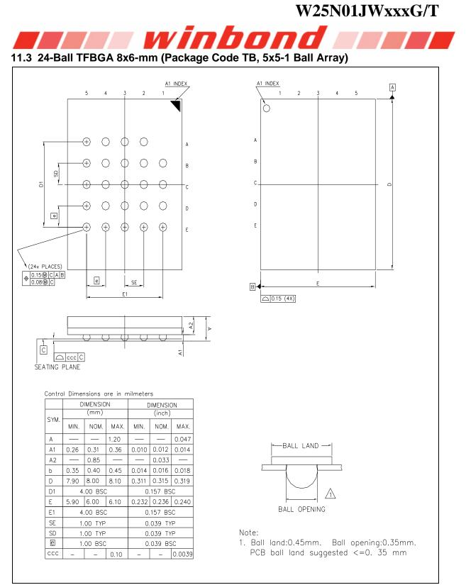
Figure 11-3 24-Ball TFBGA 8x6-mm (Package Code TB, 5x5-1 Ball Array)
