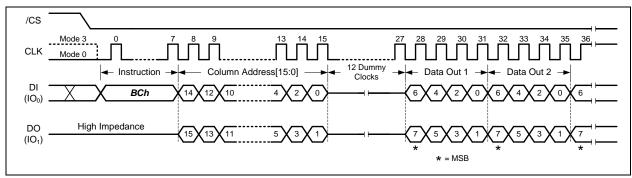
Figure 8-35 Fast Read Dual I/O with 4-Byte Address Instruction (Buffer Read Mode, BUF=1)
