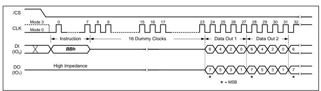
Figure 8-34 Fast Read Dual I/O Instruction (Continuous Read Mode, BUF=0)
