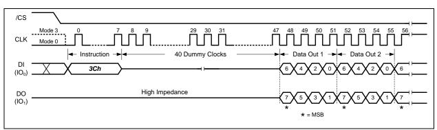
Figure 8-28 Fast Read Dual Output with 4-Byte Address Instruction (Continuous Read Mode, BUF=0)
