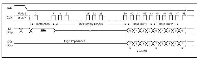
Figure 8-26 Fast Read Dual Output Instruction (Continuous Read Mode, BUF=0)
