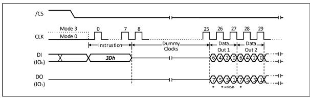
Figure 8-46 DTR Fast Read Dual Output Instruction (Continuous Read Mode, BUF=0)
