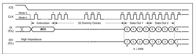
Figure 8-36 Fast Read Dual I/O with 4-Byte Address Instruction (Continuous Read Mode, BUF=0)
