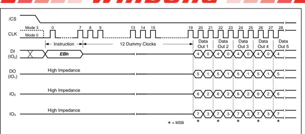
Figure 8-38 Fast Read Quad I/O Instruction (Continuous Read Mode, BUF=0)
