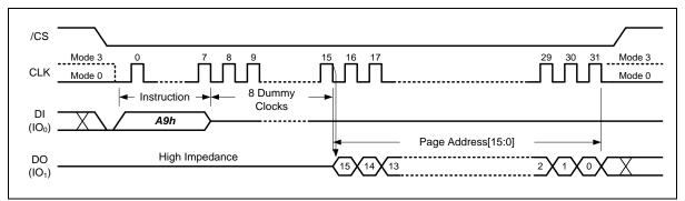
Figure 8-11 Last ECC Failure Page Address Instruction
