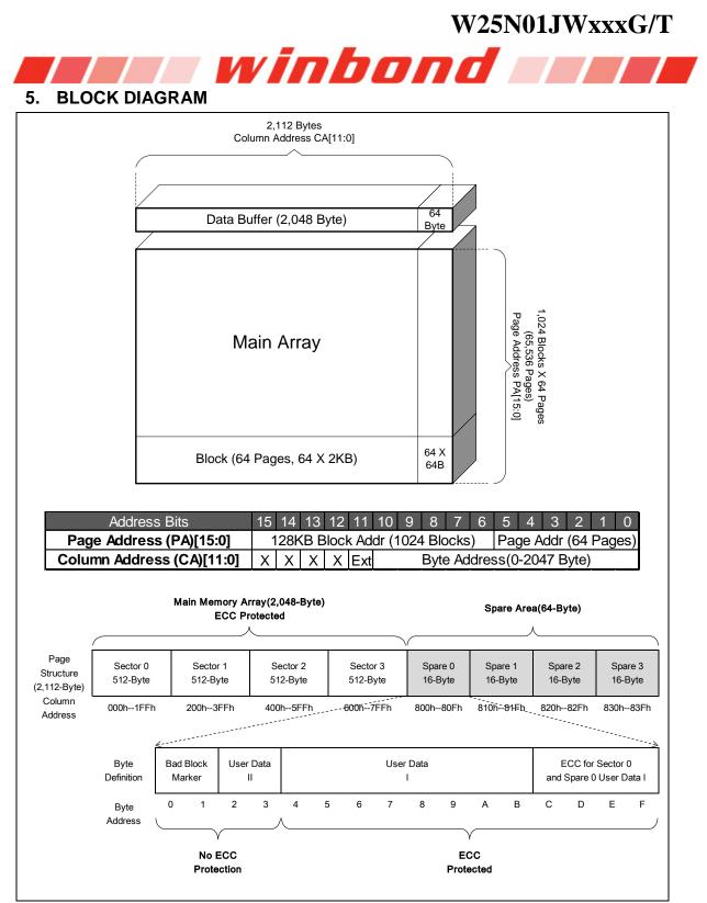
Figure 5-1 W25N01JW Flash Memory Architecture and Addressing
