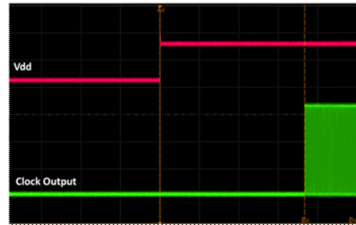
Figure 16. Startup Waveform vs. Vdd
