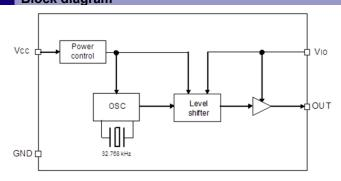
$\ensuremath{V_{\text{IO}}}$  is a power supply pin for OUT output and can also be used as an OE pin. Set  $V_{\text{IO}}$  to 0 V when setting Disable.
