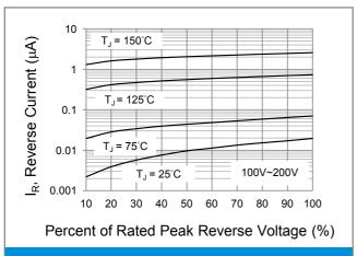
Fig.3 Typical Reverse Characteristics
