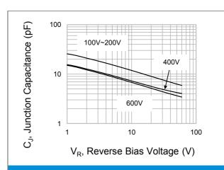
**Fig.2 Typical Junction Capacitance**
