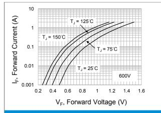
**Fig.8 Typical Forward Characteristics**
