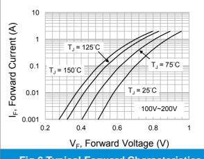
**Fig.6 Typical Forward Characteristics**
