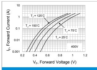
**Fig.7 Typical Forward Characteristics**
