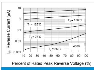
Fig.4 Typical Reverse Characteristics
