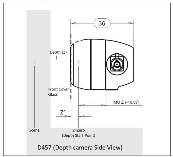
**Figure 4-4. Depth Camera Depth Start Point Reference**
