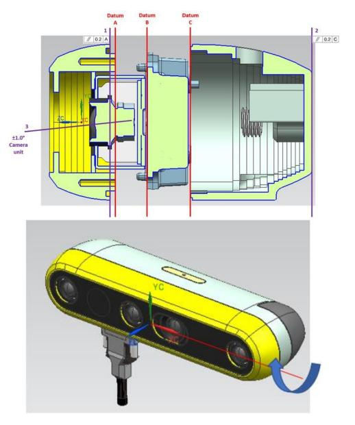
(2) Camera centerline angle relative to Rear Mounting Surface on X-Z plane (Yaw): RSS =  $\pm 1.01^{\circ}$ , worst case:  $\pm 1.19^{\circ}$
