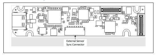
Figure 7-12. External Sensor Sync Connector Location on Depth Camera D457
