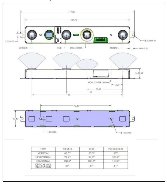
**NOTE:**  $\pm 1^{\circ}$  Optical Axis Inclination of the Stereo cameras, RGB camera, and Projector translate to the following inclination into the Rear Mounting Surface:
