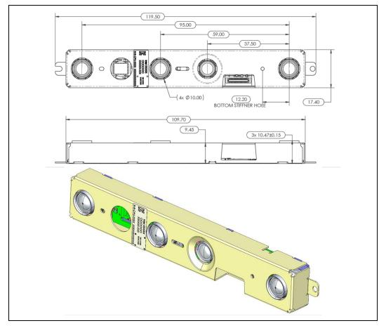
Figure 7-6. Stereo Depth Module Screw Mounting/End Mounting - D450
