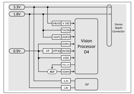
Figure 7-4. D4 Camera System Power Scheme
