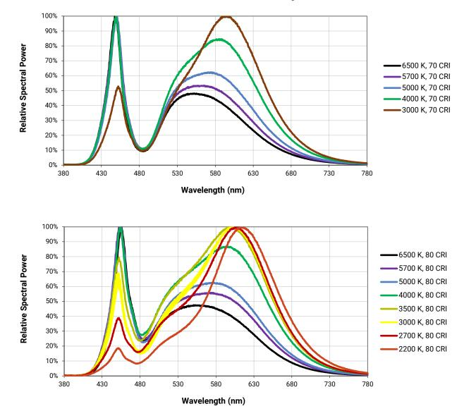
The following graphs are the result of a series of pulsed measurements at 450 mA and T<sub>1</sub> = 85 °C.
