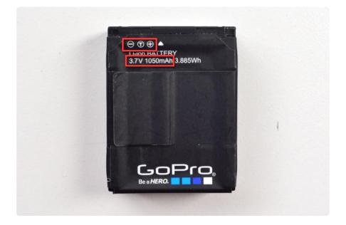
You can see its a 3.7V 1000mAh battery. That means we can charge it at 500mA max rate if we wish.
