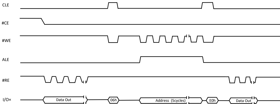
Figure 9-4 Two Plane Random Data Read (06h-E0h) Operation
