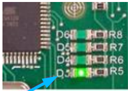
Figure 5. D3 Status LED for MCB Microcontroller
