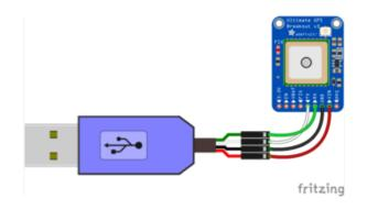
GPS Vin to USB 5V or 3V (red wire on USB console cable)
