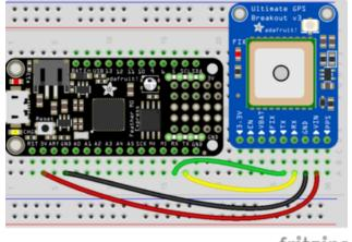
If you're using a board with hardware serial support, like this Feather M0, wire up VIN to 3.3V (since that is the logic level of the Feather M0), GND to ground, and GPS RX to Feather TX and GPS TX to Feather RX.
