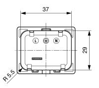
E: Quick connect terminal 6.3x0.8: 46.7 mm E: Solder terminal: 47.2 mm Version "along" (wires along to pin axis) N/PE: IDC terminals, L: quick connect or solder terminal
