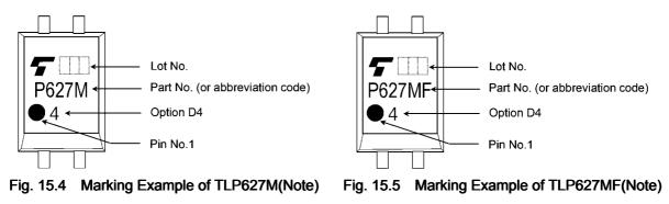
Note: The above marking is applied to the photocouplers that have been qualified according to option (D4) of EN 60747.
