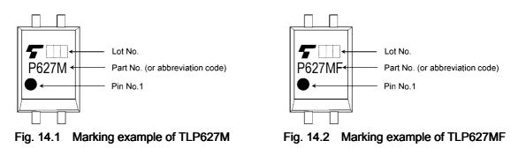
Note: A different marking is used for photocouplers that have been qualified according to option (D4) of EN 60747. See Fig.15.4 and Fig.15.5.
