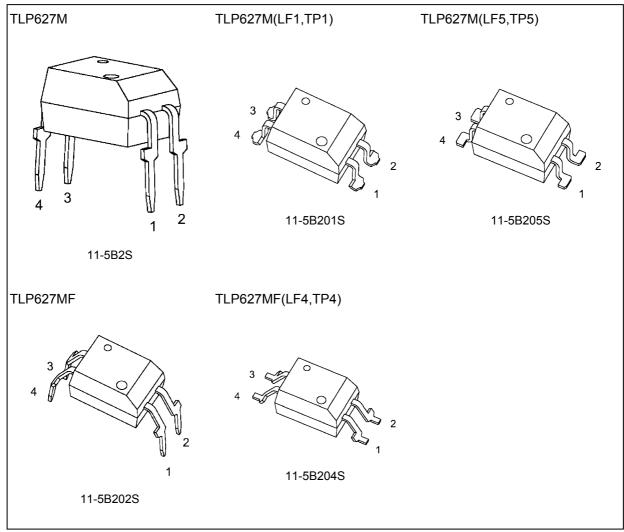
Note: Through-hole type: TLP627M, TLP627MF Lead forming option: (LF1), (LF4), (LF5) Taping option: (TP1), (TP4), (TP5)
