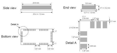
\*The pads might be slightly shorter than 1.39 mm due to PCB processing. The reduction will come from pad being pulled away from edge with up to 0.12 mm. This leaves a minimum pad lenght of 1.27 mm. The 0.1 mm distance to board edge is increase with the
