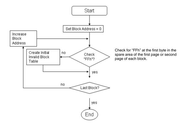
Figure 9.1 Algorithm for Bad Block Scanning
