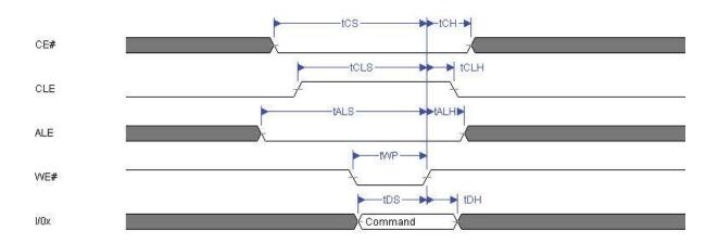
Figure 6.1 Command Latch Cycle
