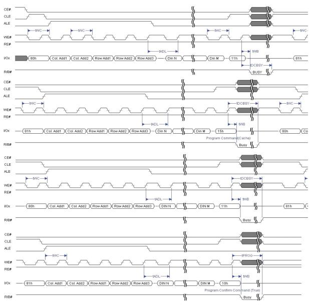
Figure 6.20 Two-Plane Cache Program Operation
