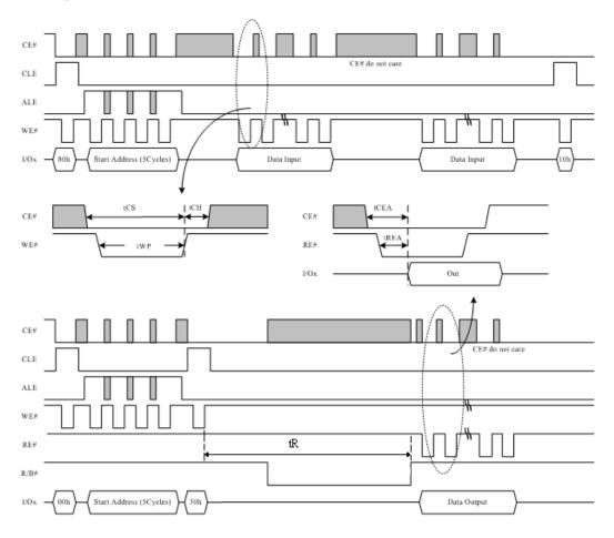
Figure 9.7 Program/Read-Operation with CE# Not-Care Operation
