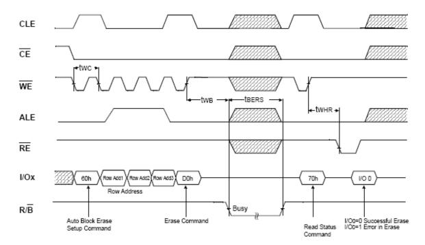
Figure 6.14. Block Erase Operation
