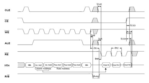
Figure 6.8 Read Operation (Intercepted by CE#)
