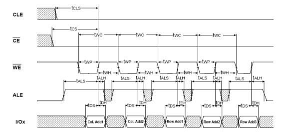
Figure 6.2 Address Latch Cycle
