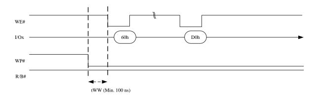
Figure 8.21 Enable/Disable Programming and Enable Erasing
