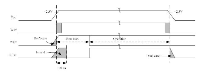
Figure 8.20 AC Waveforms for Power Transition
