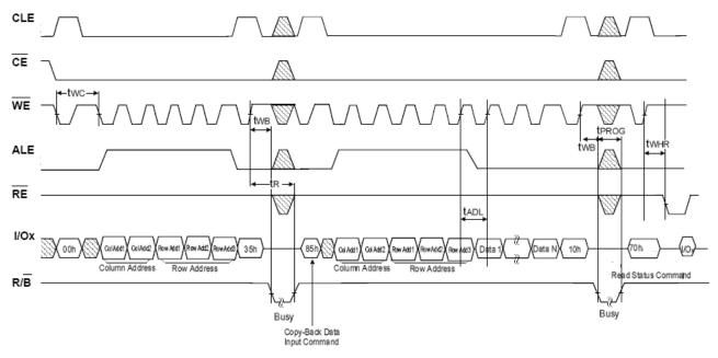
Figure 6.12 Copy-Back Operation with Random Data Input
