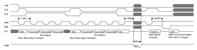
Figure 6.21 Two-Plane Block Erase Operation
