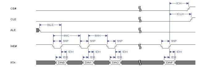
Figure 6.3 Input Data Latch Cycle
