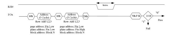
Figure 8.18 Two-Plane Block Erase
