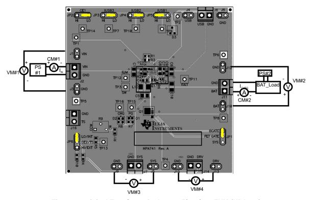
Figure 3. Original Test Setup for bq24165/166/167 EVM (HPA741)
