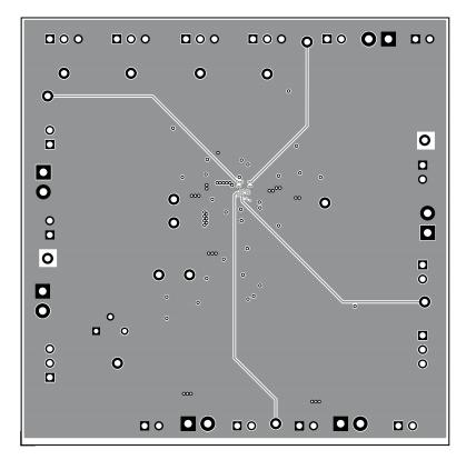
Figure 8. Second Internal Layer
