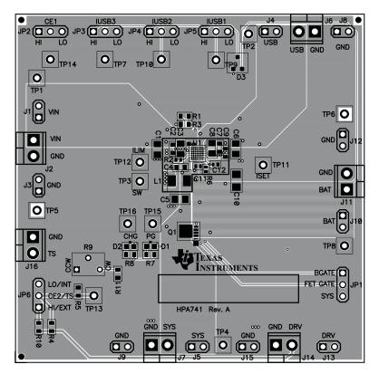
Figure 4. Top Assembly Layer
