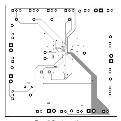
Figure 7. First Internal Layer
