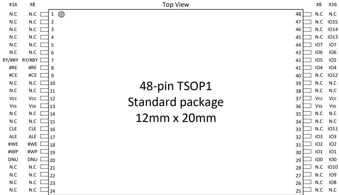
Figure 3-1 Pin Assignment 48-pin TSOP1 (Package code S)
