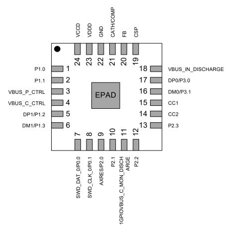
Figure 2. 24-QFN Package Pinout (Top View)
