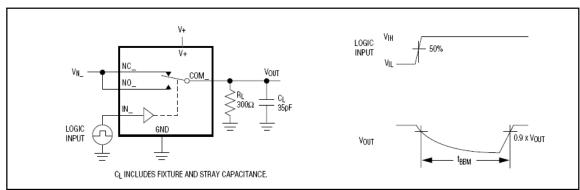
Figure 2. Break-Before-Make Interval
