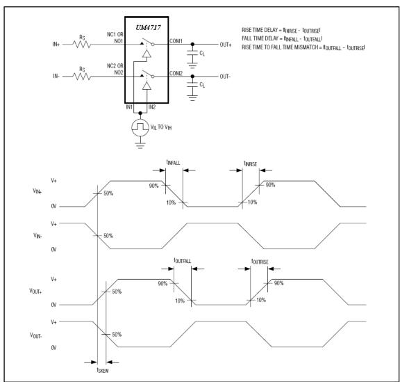
Figure 3. Output Signal Skew
