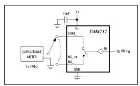
Figure 6. Channel Off/On-Capacitance
