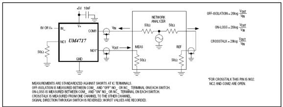
Figure 5. On-Loss, Off-Isolation, and Crosstalk
