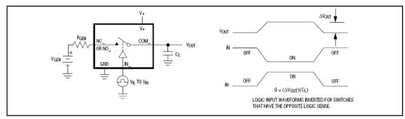
Figure 4. Charge Injection
