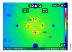
Figure 9. Infrared Image of the CN-0537 Heating Resistors
