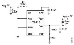
Figure 12. LT8410 Basic Connections
