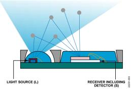
Figure 2. Backscattering of Light from ADPD188BI LEDs
