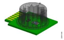
Figure 8. ADPD188BI with Smoke Chamber
