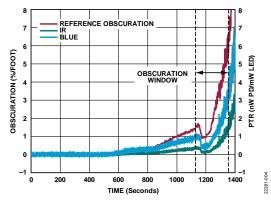
Figure 3. Smoke Profile for Burger Polyurethane Test
