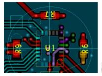
Figure 10. Placement of Heating Resistors
