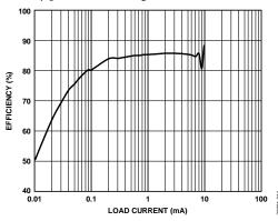
Figure 13. LT8410 Efficiency vs. Load Current Plot
