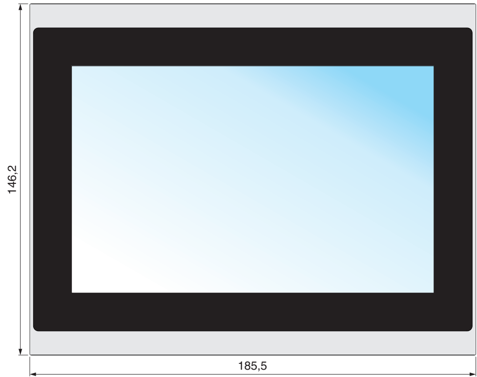
Figure 2-3 Front panel (dimensions in mm)
