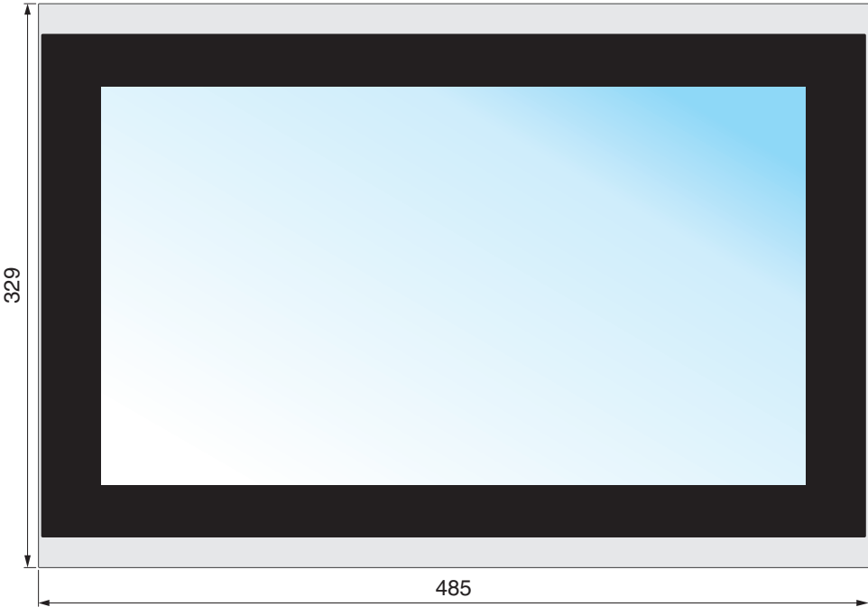
Figure 2-7 Front panel (dimensions in mm)
