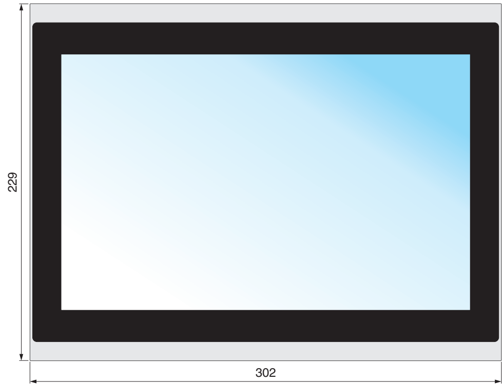
Figure 2-5 Front panel (dimensions in mm)
