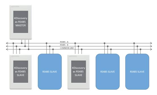
Figure 1: Typical 2-wire RS485 configuration, which includes a common ground
