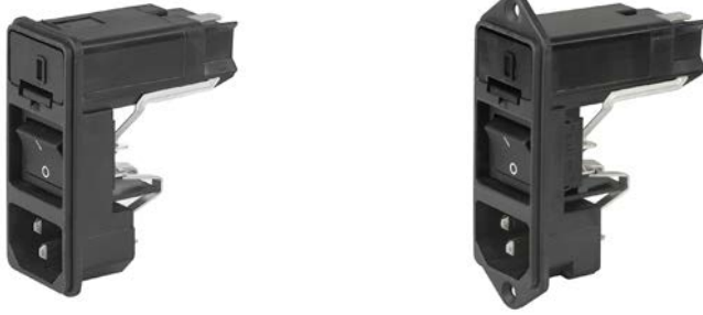
IEC connector C14 with fuse holder 1- or 2-pole Line switch 2-pole Snap-in mounting from front side Order required accessories separately
