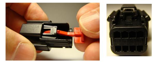
b. Confirm alignment and push on the back of the CPA until an audible and tactile click is heard and felt
