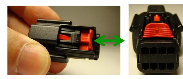
d. CPA properly installed and in the proper position
