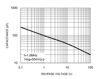
Fig.2 Typical Junction Capacitance
