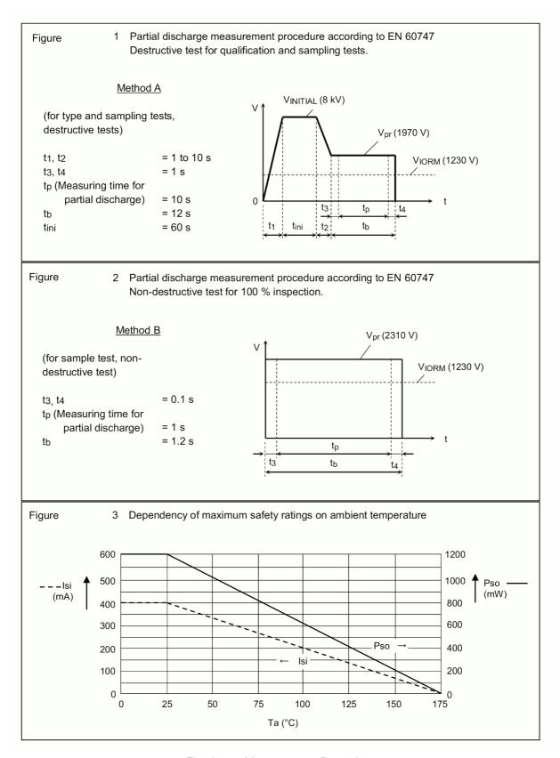
Fig. 17.5 Measurement Procedure
