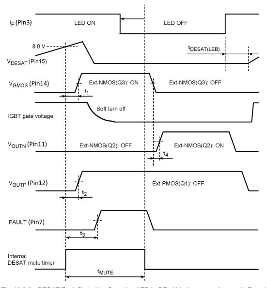
Fig. 13.2.2 DESAT Fault State (the Case that LED is Off within the t<sub>MUTE</sub>: Automatic Reset)
