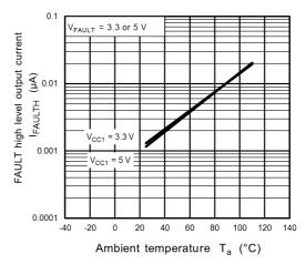
Fig. 13.3.28 I<sub>FAULTH</sub> - T<sub>a</sub>
