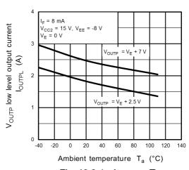
Fig. 13.3.4 I<sub>OUTPL</sub> - T<sub>a</sub>
