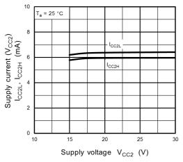
Fig. 13.3.21 I<sub>CC2H</sub>, I<sub>CC2L</sub> - V<sub>CC2</sub>
