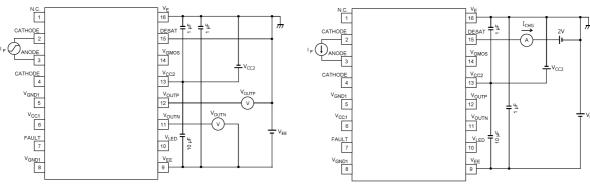
Fig. 13.1.15 I<sub>FHL</sub>, I<sub>FLH</sub> Test Circuit
