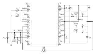
Fig. 13.1.19 CM<sub>H</sub> Refer to V<sub>E</sub> Test Circuit (Gate Output: OFF)
