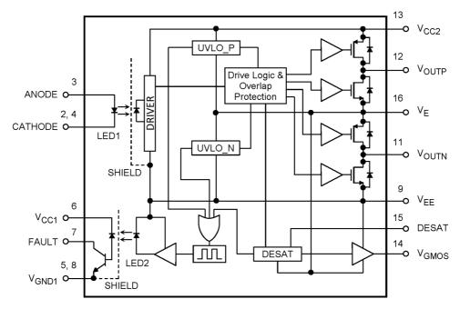
Note: A  $10\mu F$  bypass capacitor must be connected between pins 9 and 13, and A  $1\mu F$  bypass capacitor must be connected between pins 13 and 16, and pins 9 and 16.
