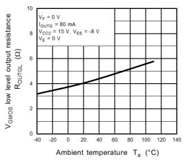
Fig. 13.3.18 R<sub>OUTGL</sub> - T<sub>a</sub>
