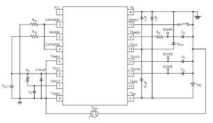
Fig. 13.1.20 CM<sub>L</sub> Refer to V<sub>E</sub> Test Circuit (Gate Output: ON)
