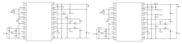
Fig. 13.1.17  $t_{pLH}$ ,  $t_{pHL}$ ,  $t_{NLH}$ ,  $t_{NHL}$ ,  $t_{DP}$ ,  $t_{DN}$ ,  $t_{PR}$ ,  $t_{NR}$ ,  $t_{NF}$  Test Circuit
