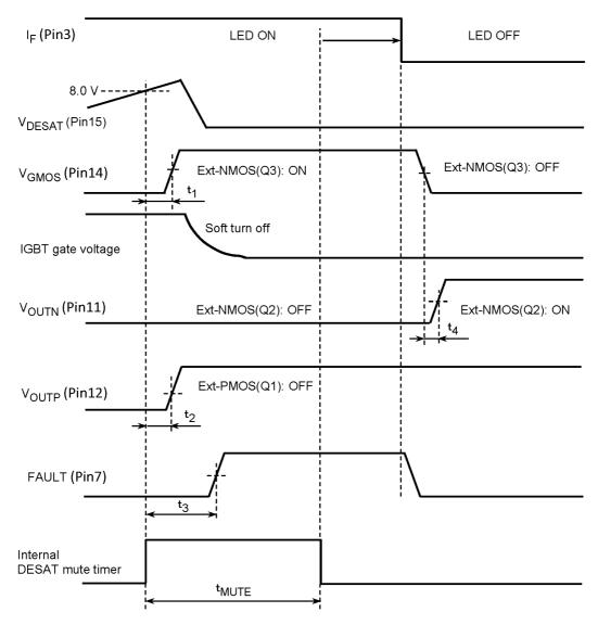
Fig. 13.2.3 DESAT Fault State (the Case that LED is Off after t<sub>MUTE</sub>: Reset by LED Trigger)
