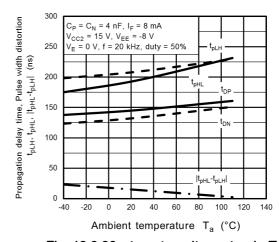
Fig. 13.3.30  $t_{pLH}$ ,  $t_{pHL}$ ,  $|t_{pHL} - t_{pLH}| - T_a$
