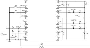
Fig. 13.1.22 CM<sub>L</sub> Refer to V<sub>GND1</sub> Test Circuit (Fault Output: LOW)
