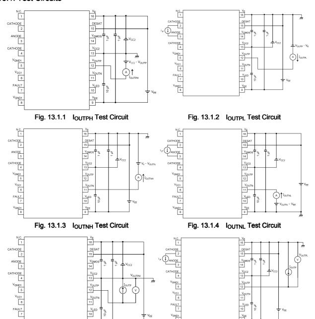
Fig. 13.1.5 Voutph, Routph Test Circuit
