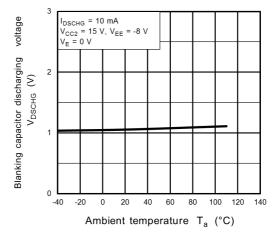
Fig. 13.3.24 V<sub>DSCHG</sub> - T<sub>a</sub>
