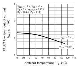
Fig. 13.3.27 I<sub>FAULTL</sub> - T<sub>a</sub>
