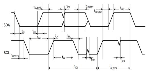
The following table provides the I<sup>2</sup>C slave timing parameters for the ATWINC3400 IC.
