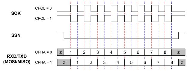
The SPI timing is provided in the following figure and table.
