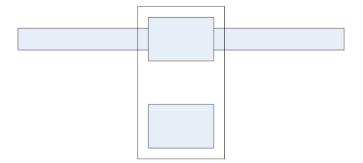
The following figure shows a stub route to the capacitor pad. This should be avoided, as it adds additional impedance in series with the capacitor.
