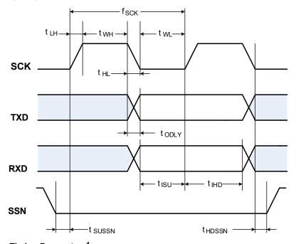
Table 8-5. SPI Slave Timing Parameters<sup>1</sup>
