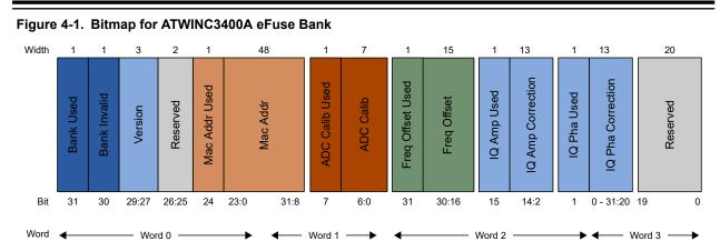
**Note:** The bit map has been updated with bit fields IQ Amp correction and IQ Pha Correction fields from FW version 1.4 onwards. Previously these bit fields were reserved for future use. For customers using FW older than 1.4, IQ Amp correction and IQ Pha Correction bit fields will not be used by the FW.
