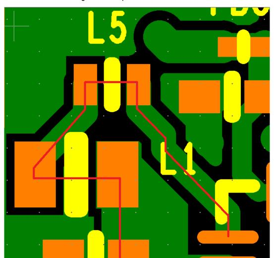
Figure 13-2. Placement and Routing of PMU Components
