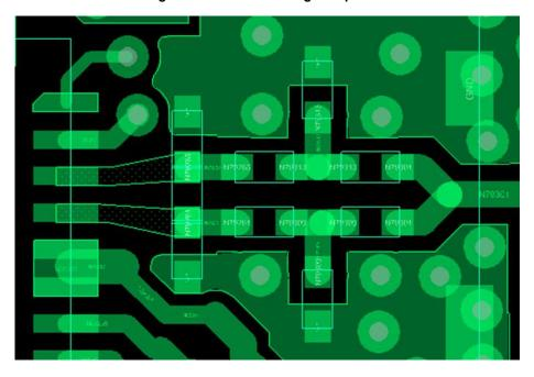
Figure 13-1. Placement and Routing of Balun and Matching Components
