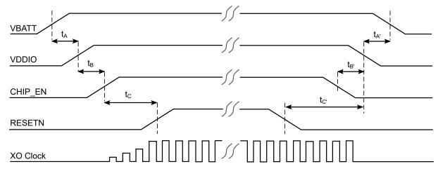
The following table provides power-up/down sequence timing parameters.
