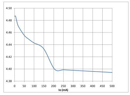
Figure 10. Buck Boost Load Regulation,  $V_{IN}$  = 3.6 V,  $V_{O}$  = 4.5 V, PFM Mode
