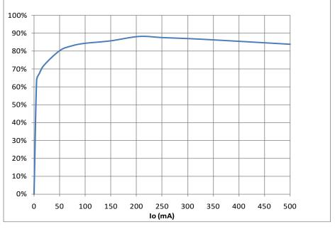
Figure 8. Buck Boost Efficiency,  $V_{IN}$  = 3.6 V,  $V_{O}$  = 4.5 V
