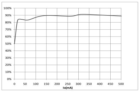
Figure 9. Buck Boost Efficiency,  $V_{IN}$  = 3.6 V,  $V_{O}$  = 2.8 V
