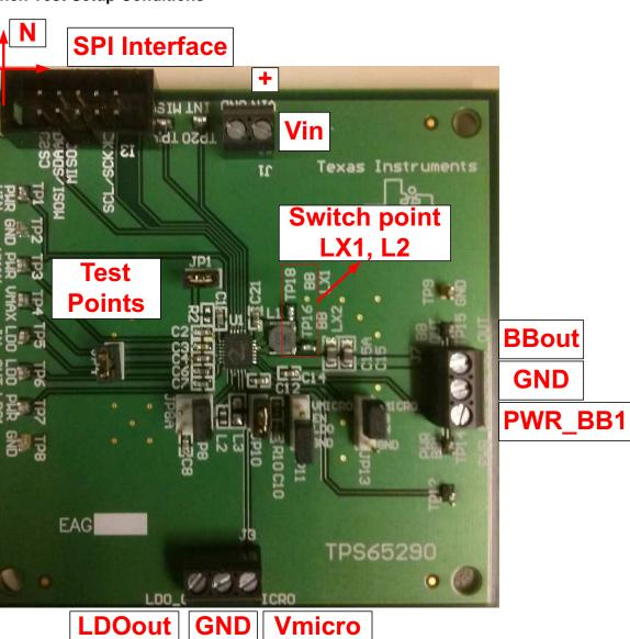
Figure 18. Headers Description and Jumper Placement
