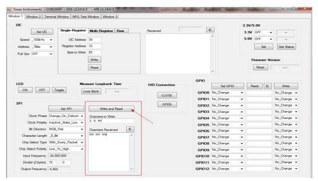
Figure 5. Unlock the USB2ANY
