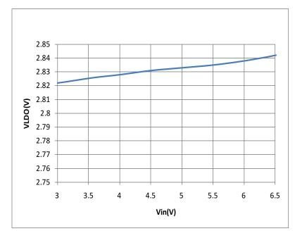
Figure 11. Buck Boost Line Regulation,  $V_o = 2.8 V$ ,  $I_o = 5 mA$
