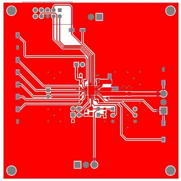
Figure 14. Board Layout (Top Layer)
