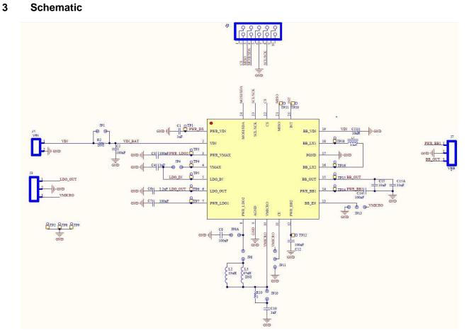
Figure 12. TPS65290 Schematic
