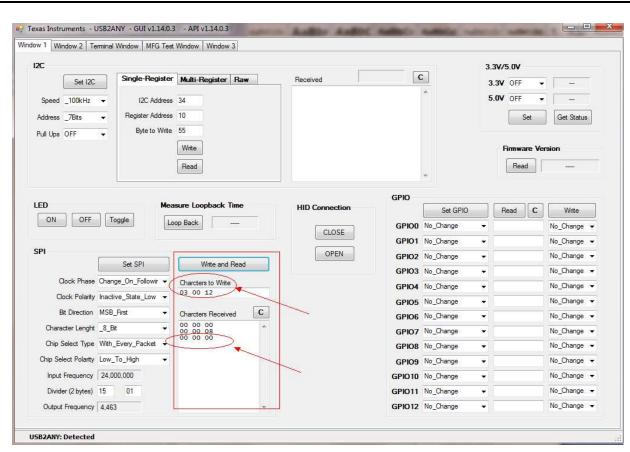
Figure 7. Write the Register
