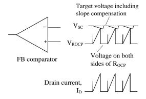
Figure 9-6 Drain current, I<sub>D</sub>, and FB comparator operation in steady operation
