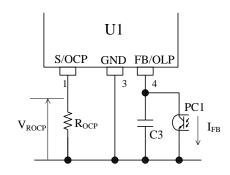
Figure 9-5 FB/OLP pin peripheral circuit
