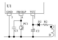
Figure 9-12 FB/OLP pin peripheral circuit
