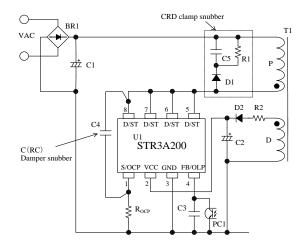
Figure 10-1 The IC peripheral circuit
