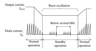
Figure 9-8 Auto Standby mode timing
