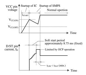
Figure 9-4  $V_{\text{CC}}$  and  $I_{\text{D}}$  behavior during startup
