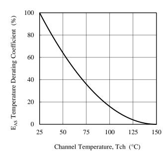
Figure 3-1 SOA Temperature Derating Coefficient Curve
