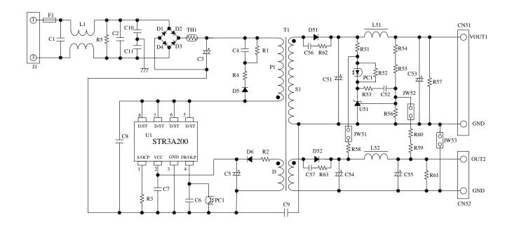
Figure 11-2 Circuit schematic for PCB circuit trace layout
