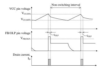
Figure 9-13 OLP operational waveforms
