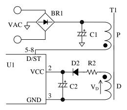
Figure 9-1 VCC pin peripheral circuit
