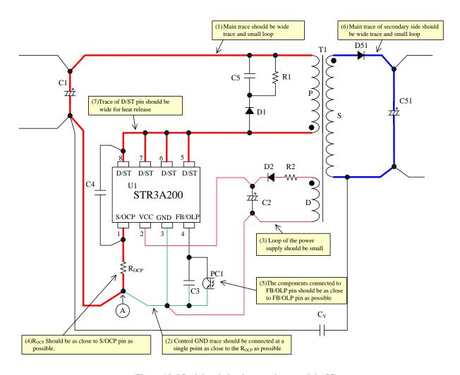
Figure 10-5 Peripheral circuit example around the IC
