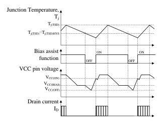
Figure 9-15 TSD operational waveforms
