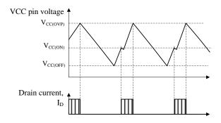
Figure 9-14 OVP operational waveforms
