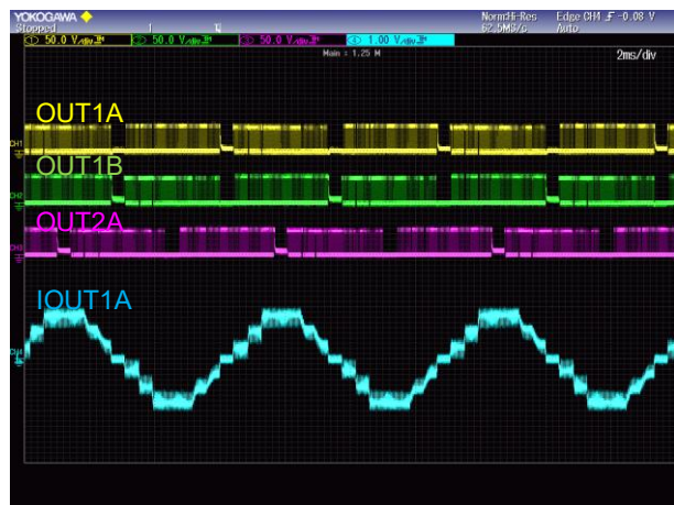
Figure 17. QUARTER STEP ( CLK : 2400Hz )
