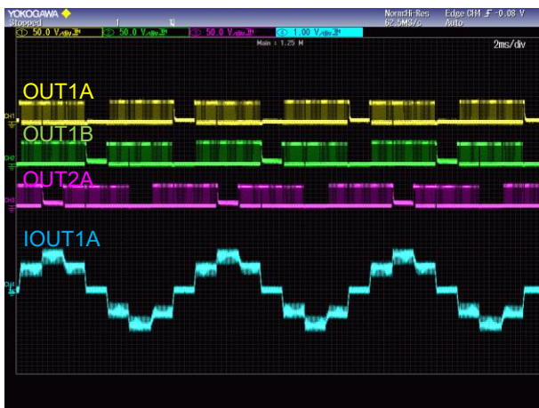
Figure 16. HALF STEP B ( CLK : 1200Hz )
