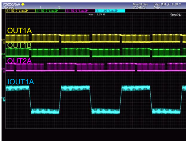
Figure 14. FULL STEP ( CLK : 600 Hz )
