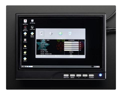
Picture Mode - Standard, Personal, Vivid, Movie Contrast - Adjust the contrast Brightness - Adjust the brightness Color - Adjust the color Tint - Adjust the tint Sharpness - Adjust the sharpness Color Temp - Normal, Cool, Warm
