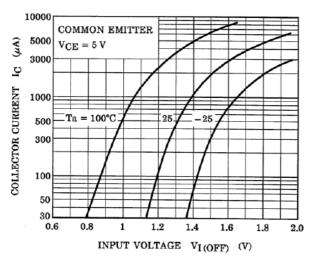
Fig. 10.9 RN1303 I<sub>C</sub>-V<sub>I(OFF)</sub>
