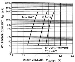
Fig. 10.8 RN1302 I<sub>C</sub>-V<sub>I(OFF)</sub>
