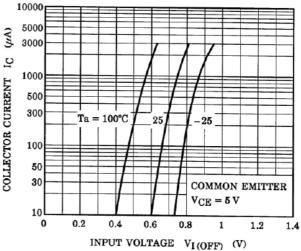
Fig. 10.12 RN1306 I<sub>C</sub>-V<sub>I(OFF)</sub>
