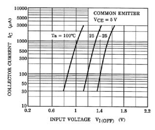
Fig. 10.7 RN1301 I<sub>C</sub>-V<sub>I(OFF)</sub>
