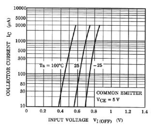
Fig. 10.11 RN1305 I<sub>C</sub>-V<sub>I(OFF)</sub>
