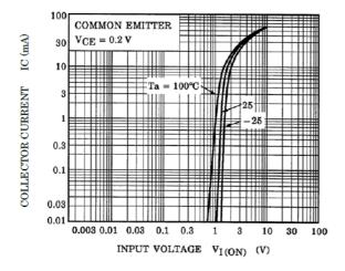
Fig. 10.1 RN1301 I<sub>C</sub>-V<sub>I(ON)</sub>
