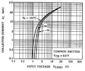
Fig. 10.3 RN1303 I<sub>C</sub>-V<sub>I(ON)</sub>
