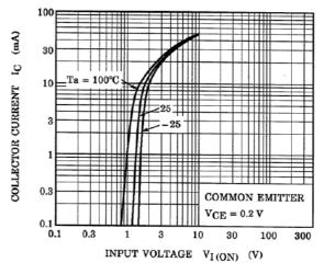
Fig. 10.2 RN1302 I<sub>C</sub>-V<sub>I(ON)</sub>
