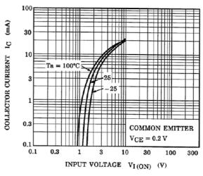
Fig. 10.4 RN1304 I<sub>C</sub>-V<sub>I(ON)</sub>
