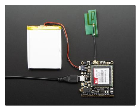
Then press the small KEY button next to the battery & cell antenna for 5 seconds. Then the computer will recognize a multi-type USB connection. Install the drivers () There are 4 devices created
