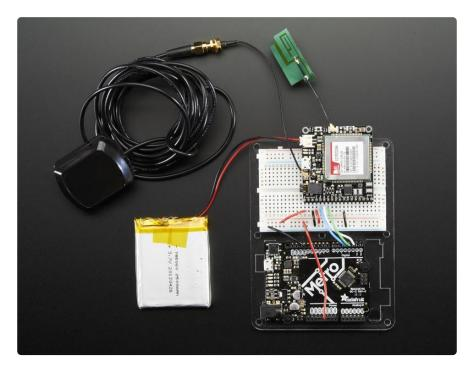
Check polarity for the battery! Snap the uFL connector on, it will click when placed properly
