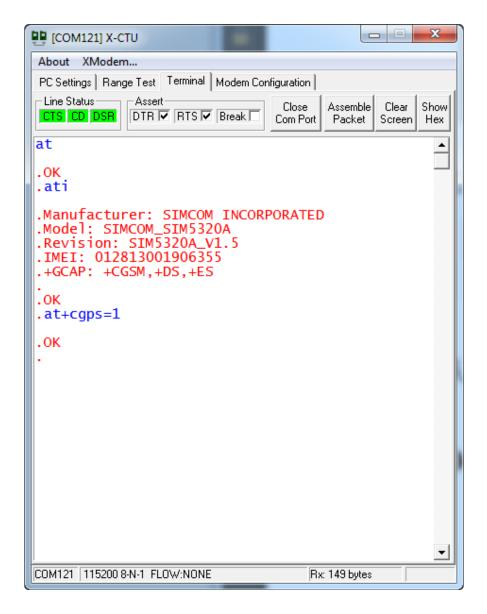
If you turn on the gps with the at+cgps=1 command in the AT serial port you can then connect to the NMEA COM port and see GPS NMEA data
