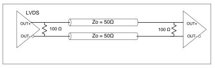
Figure 16. LVDS Double DC Termination
