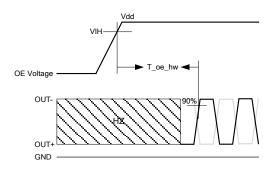
Figure 8. Hardware OE Enable Timing
