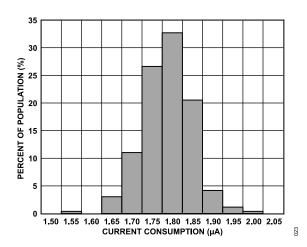
Figure 23. Current Consumption at 25°C, Normal Mode, ODR = 100 Hz,  $V_S = 2 V$
