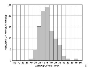
Figure 5. X-Axis Zero g Offset at 25°C,  $V_S = 2 V$
