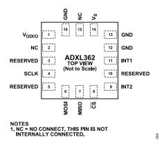
Figure 4. Pin Configuration (Top View)
