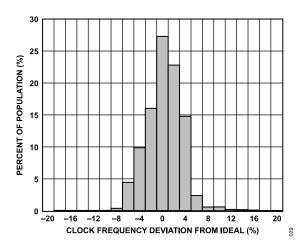
Figure 29. Clock Frequency Deviation from Ideal at 25°C,  $V_S$  = 2 V
