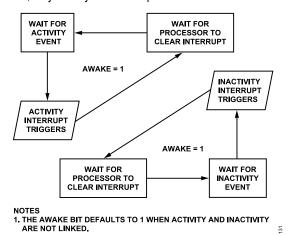
Figure 31. Flowchart Illustrating Activity and Inactivity Operation in Default
