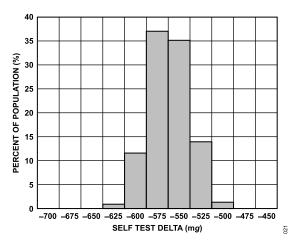
Figure 21. Y-Axis Self Test Response at 25°C, V<sub>S</sub> = 2 V
