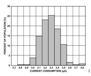
Figure 24. Current Consumption at 25°C, Low Noise Mode, ODR = 100 Hz,  $V_S$  = 2 V
