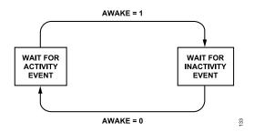
Figure 33. Flowchart Illustrating Activity and Inactivity Operation in Loop
