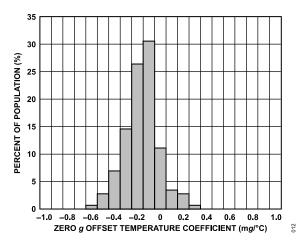
Figure 12. Y-Axis Zero g Offset Temperature Coefficient, V<sub>S</sub> = 2 V
