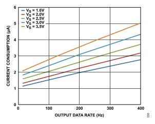
Figure 30. Current Consumption vs. Output Data Rate at Several Supply Voltages
