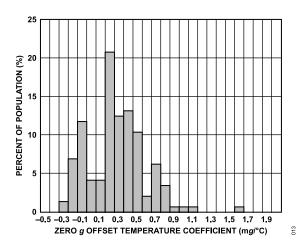
Figure 13. Z-Axis Zero g Offset Temperature Coefficient, V<sub>S</sub> = 2 V
