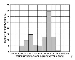
Figure 28. Temperature Sensor Scale Factor,  $V_S = 2 V$
