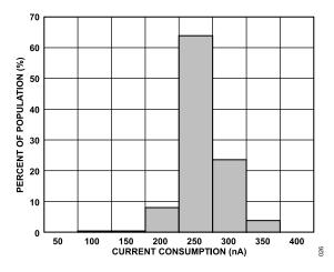
Figure 26. Current Consumption at 25°C, Wake-Up Mode,  $V_S$  = 2 V
