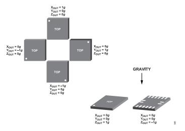
Figure 52. Output Response vs. Orientation to Gravity
