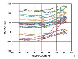
Figure 16. Z-Axis Zero g Offset vs. Temperature— 16 Parts Soldered to PCB, ODR = 100 Hz,  $V_S$  = 2 V
