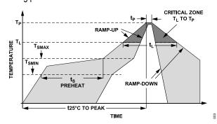
Figure 3. Recommended Soldering Profile
