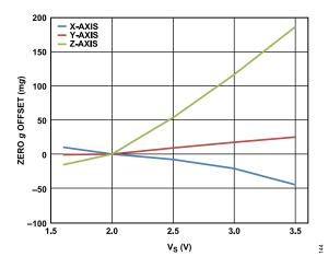
Figure 50. 0 g Offset vs. Supply Voltage
