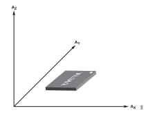
Figure 51. Axes of Acceleration Sensitivity (Corresponding Output Increases When Accelerated Along the Sensitive Axis)
