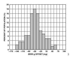
Figure 7. Z-Axis Zero g Offset at 25°C,  $V_S = 2 V$
