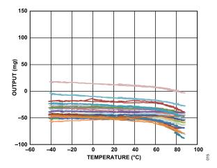
Figure 15. Y-Axis Zero g Offset vs. Temperature— 16 Parts Soldered to PCB, ODR = 100 Hz,  $V_S$  = 2 V
