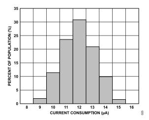
Figure 25. Current Consumption at 25°C, Ultralow Noise Mode, ODR = 100 Hz,  $V_S$  = 2 V
