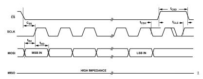
Figure 41. Timing Diagram for SPI Receive Instructions
