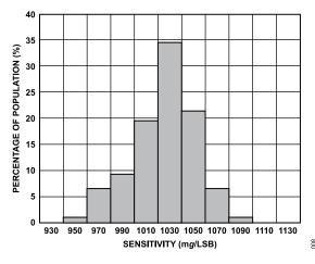
Figure 8. X-Axis Sensitivity at 25°C,  $V_S = 2 V$ ,  $\pm 2 g$  Range
