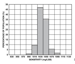
Figure 9. Y-Axis Sensitivity at 25°C,  $V_S = 2 V$ ,  $\pm 2 g$  Range
