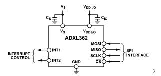
Figure 46. Recommended Bypass Capacitors
