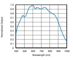
Fig. 14 - White Channel Spectral Response
