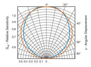
Fig. 12 - Relative Sensitivity vs. Angular Displacement (ALS)
