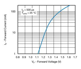
Fig. 7 - Forward Current  $I_F = f(V_F)$  for LED
