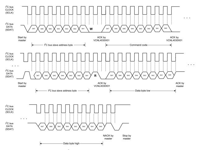
Fig. 4 - I<sup>2</sup>C Bus Timing for Receiving Word Command Format
