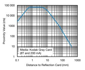
Fig. 15 - Proximity Value vs. Distance to Reflecting Card
