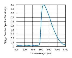
Fig. 6 - Normalized Spectral Response (PS channel)
