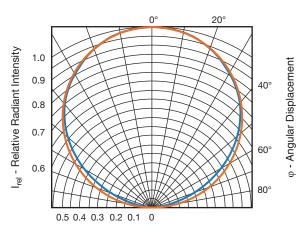
Fig. 10 - Relative Radiant Intensity Emitter vs. Angular Displacement
