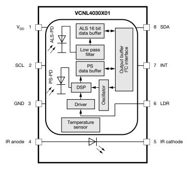
Fig. 1 - Detailed Block Diagram
