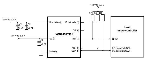
Fig. 16 - Circuitry with Two Separate Power Supply Sources
