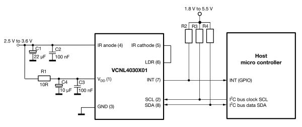
Fig. 18 - Circuitry with Just One Common Power Supply Source
