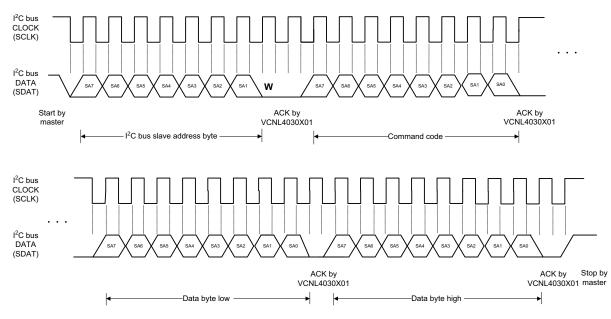
Fig. 3 - I<sup>2</sup>C Bus Timing for Sending Word Command Format
