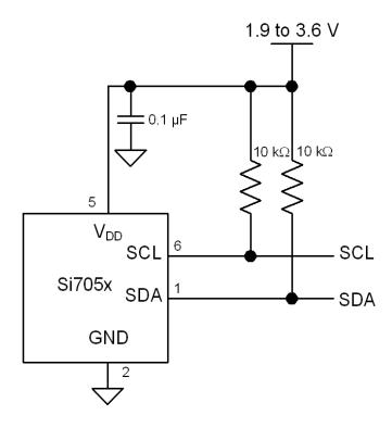
Figure 2. Typical Application Circuit for Temperature Measurement
