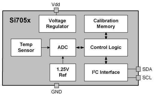
Figure 3. Si705x Block Diagram
