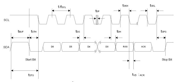
Figure 1. I<sup>2</sup>C Interface Timing Diagram
