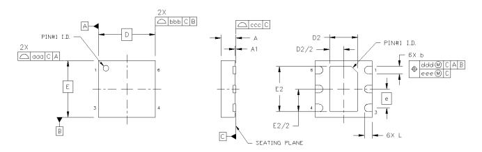
Figure 10. 3x3 6-pin DFN
